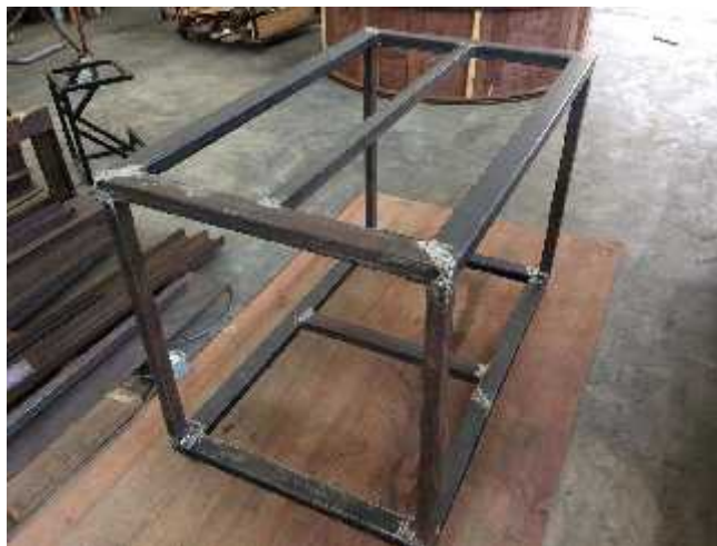
Figure 9: Iron rack/stand for placing dough fermenting basin or trays (50*70 cm width and length, 90 cm height and square hollow iron bar of 4*4 cm and 2 mm thickness)
