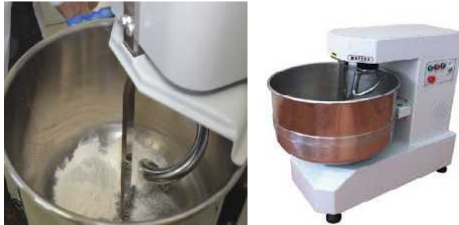
Figure 2: Spiral dough mixer (60 kg capacity)
