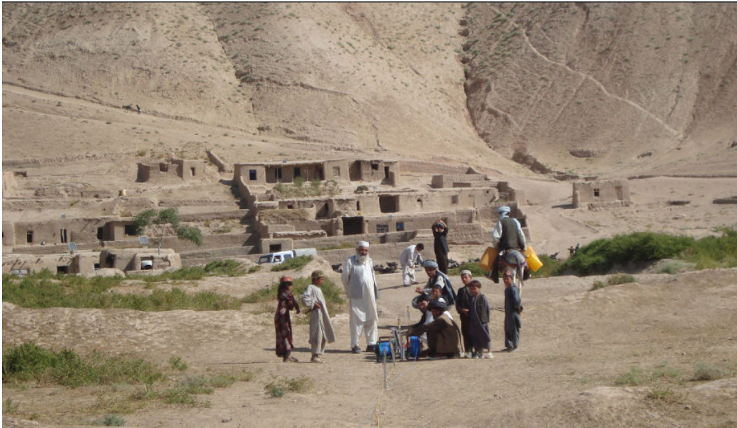
Fig. 22, Applying vertical electrical sounding (VES) in the field.
