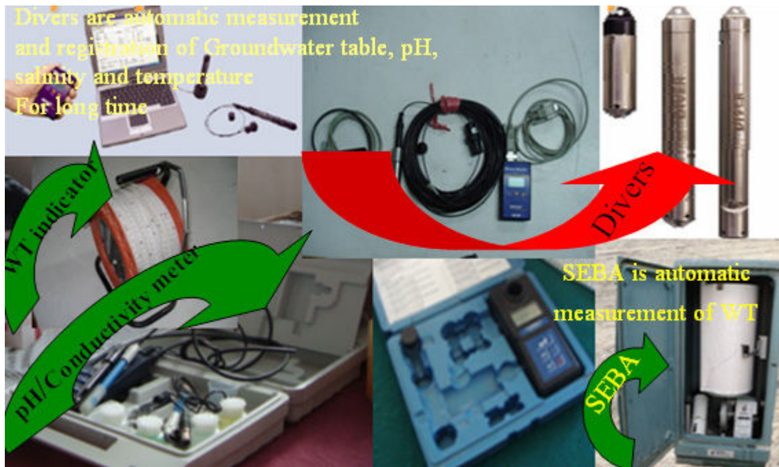
Figure 2 Water Table and Physical parameters measurement devices
