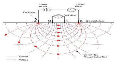
**Figure 4 Vertical Electrical Sounding Method**
