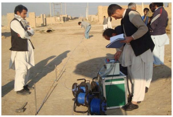
Figure 1 Recording VES profile field data using SYSCAL Pro resistivty meter
