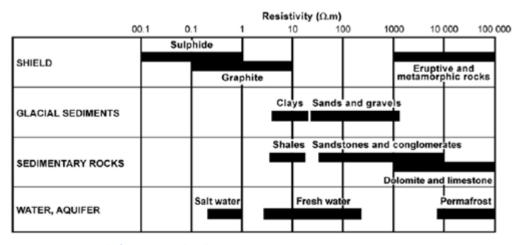
Figure 5 Resistivity scale for water and rocks
