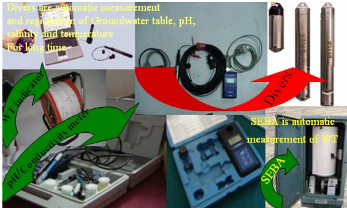
Figure 2, Water table and physical parameters measurement devices
